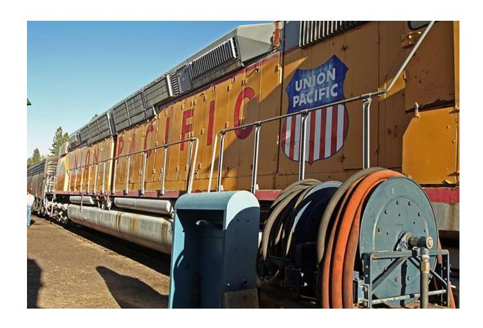
Union Pacific Railroad constructed the Centennial locomotives the largest diesel-electric engines ever built. They actually were made up of two engines on one frame and they operated in freight service from 1969 to 1984. Thirteen of these massive machines are in museums, with one, number 6946, at the Western Pacific Railroad Museum at Portola.
