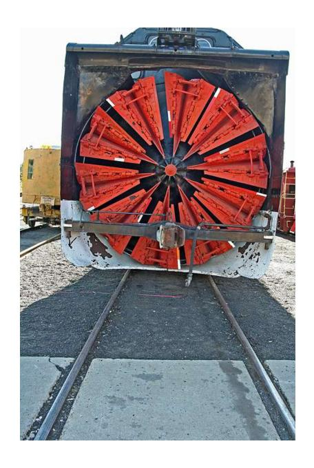
One of the locomotives is equipped with a rotary snow plow on the front. Snow levels over the Sierra Nevada mountain range can exceed six feet or more and equipment like this is needed to keep the tracks clear.
